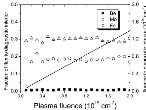
**FIGURE 3.** Fluence entering the diagnostic beyond the first mirror (solid line, right axis) and its composition (symbols, left axis). The remainder of the composition is DT
