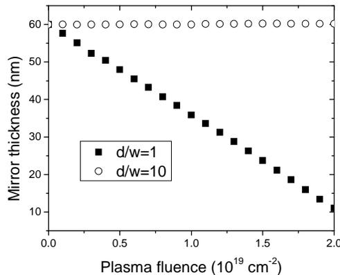
**FIGURE 4.** Erosion of the first mirror vs. fluence for a short ( $d/w=1$ ) and a long ( $d/w=10$ ) slit.
