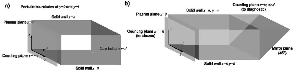
**FIGURE 1.** Geometries used in the simulation of a) a gap between two tiles, and b) the slit of an optical diagnostic
