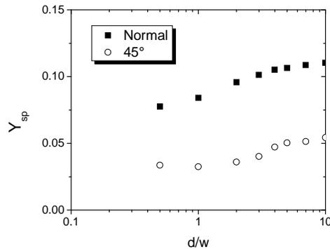
**FIGURE 1.** Total sputtering yield of gap material as a function of gap depth, for a plasma plane parallel to the opening and tilted  $45^\circ$ .
