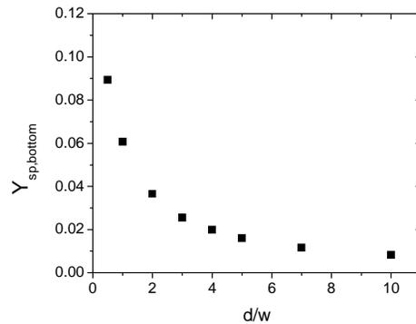
**FIGURE 2.** Total sputtering yield of gap material as a function of gap depth, for a plasma plane parallel to the opening and tilted  $45^\circ$ .
