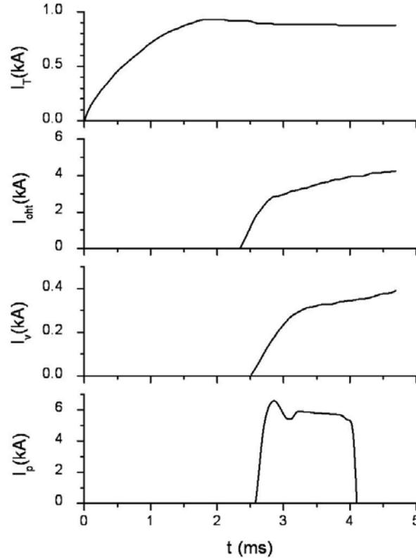
**FIGURE 2.** Set of signals used for the reconstruction of the magnetic field surfaces in a plasma discharge lasting approximately 1500  $\mu\text{s}$ . These are, from top to bottom, the toroidal field coils current, the ohmic heating coil current, the vertical field coils current, and the plasma current.
