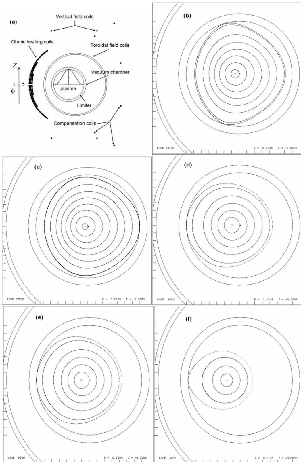
**FIGURE 3.** (a) Coil arrangement for the NOVILLO tokamak (b-f) Reconstruction for surfaces at 50, 150, 400, 700 and 1450  $\mu$ s, for the discharge shown in Fig. 1.
