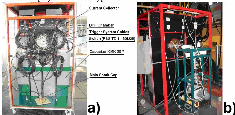
**FIGURE 2.** The photo of DPF 6.0 device: back (a); front face (b).
