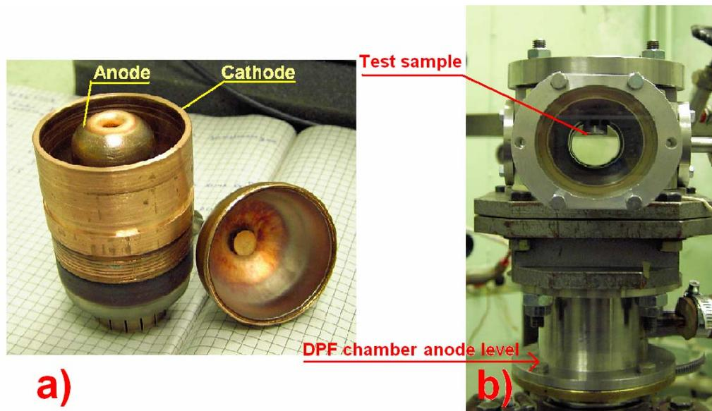
**FIGURE 4.** The photo of the DPF chamber, opened in order to take opportunity to connect target unit with the chamber (a); (b) the target unit with the test sample, connected to DPF chamber. PF 5M device
