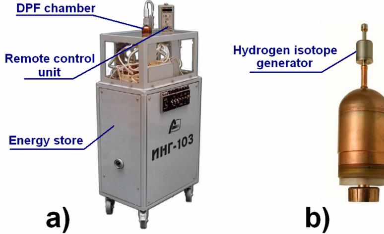
**FIGURE 1.** The photo of ING-103 neutron pulse generator (a); neutron DPF chamber (b).
