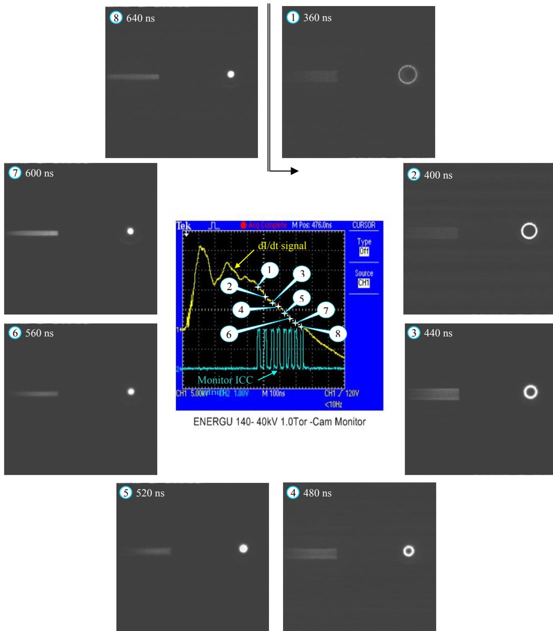
**FIGURE 2,** Side – Front simultaneous pictures and  $di/dt$  signal vs ICC monitor pulses.  $V_0 = 40$  kV, 1.0 torr, 5ns exposure time, 40 ns delay between pictures.
