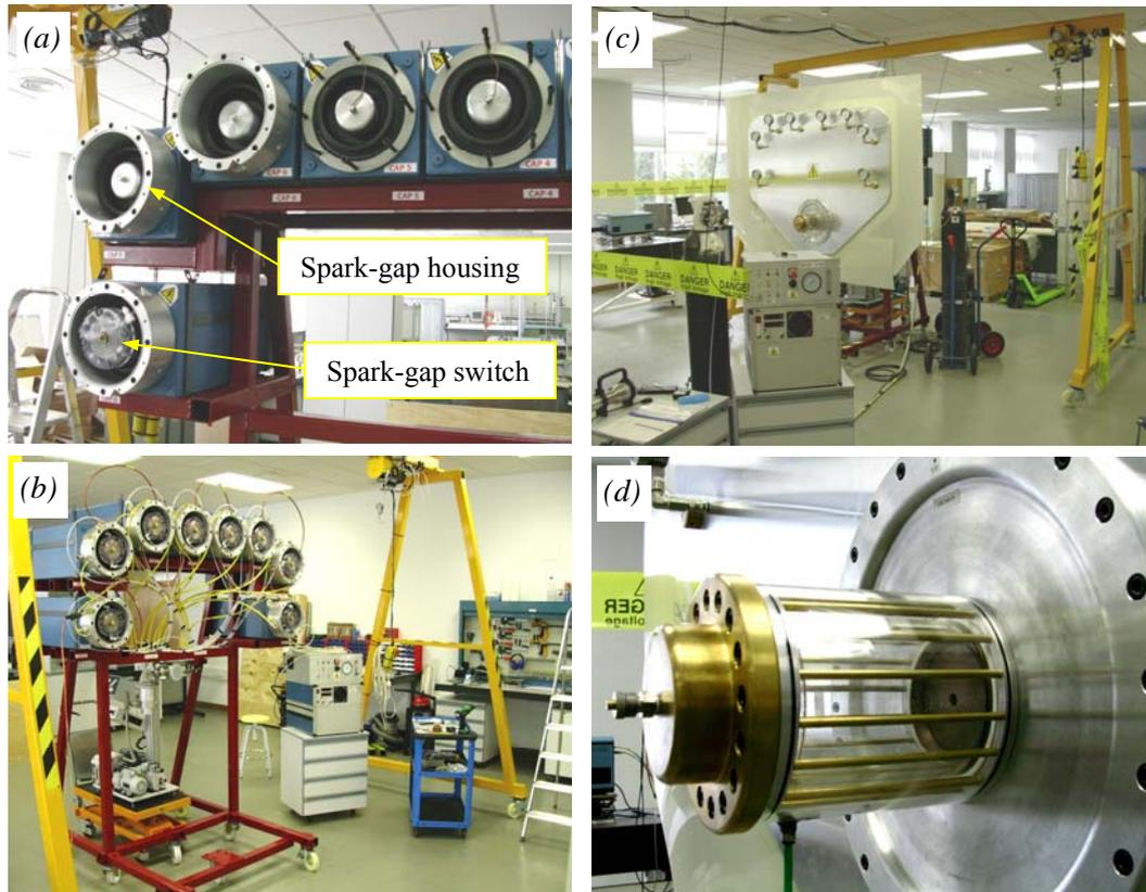
**FIGURE 1**, Different stages of the z-pinch machine development. (a) View of the spark-gap housing and switches mounting. (b) All Switching system ready for mounting the transmission line. (c): The machine full mounted and ready for firing. (d) A discharge chamber close-up.
