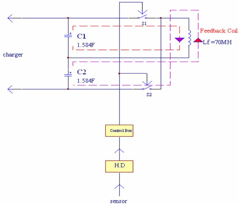
**FIGURE 3.** Block Diagram of Feedback System
