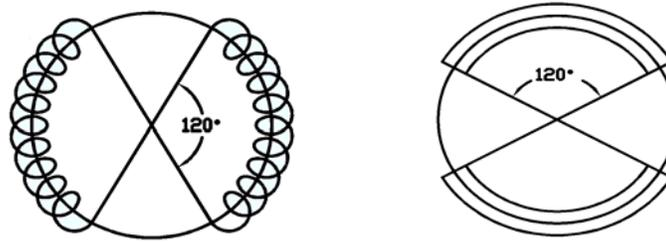
**FIGURE 1.** Schematic diagram of cosine and saddle coil of IR-T1 tokamak
