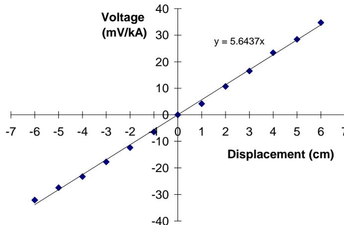
**FIGURE 2.** Cosine coil output as a function of horizontal displacement.
