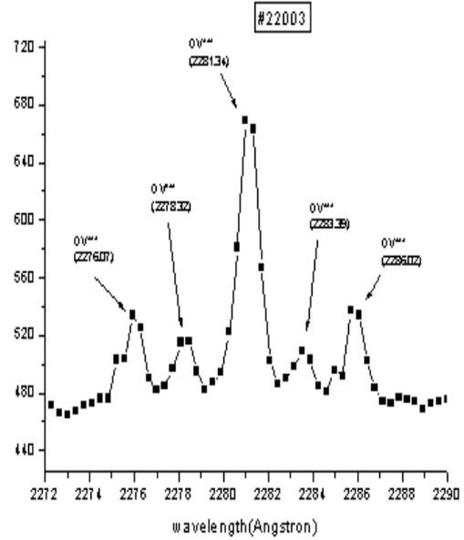
FIGURE 2. Third order OV line at 228.134 nm
