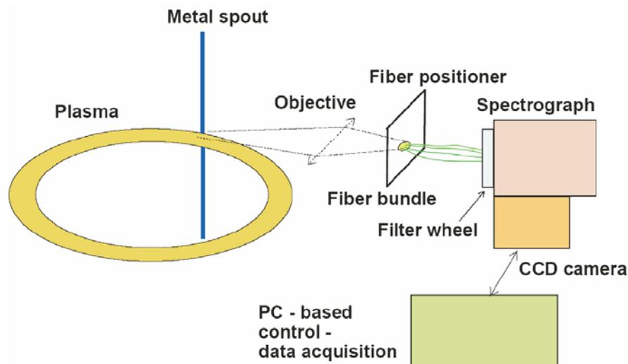
FIGURE 1. Schematic of ISTTOK's imaging spectrograph diagnostic<sup>5</sup>
