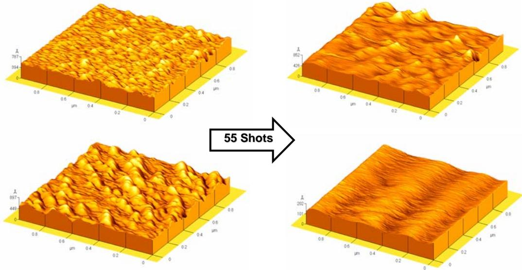
**FIGURE 2.** Changes in roughness at two different positions of the sample with respect to plasma core. Below one is closer to plasma core. Left figures are before discharges and right figures are after discharge.
