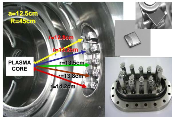
**FIGURE 1.** An array of samples installed inside the tokamak vessel.
