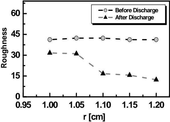
**FIGURE 3.** Profile of comparing roughness of samples before discharge and after discharges, where,  $r$  (normalized) is the position of samples with respect to plasma core.
