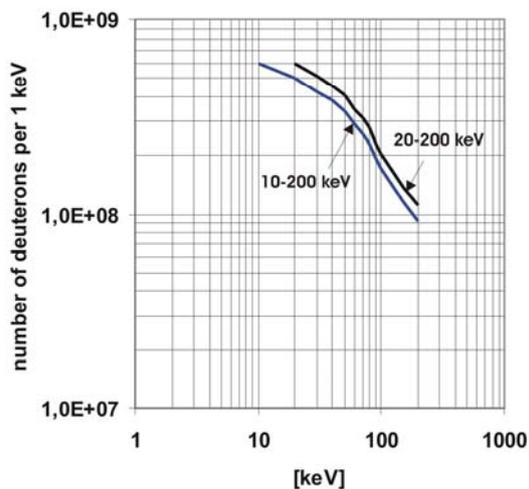
**FIGURE 4:** Spectral distribution of energy of deuterons produced observed neutrons
