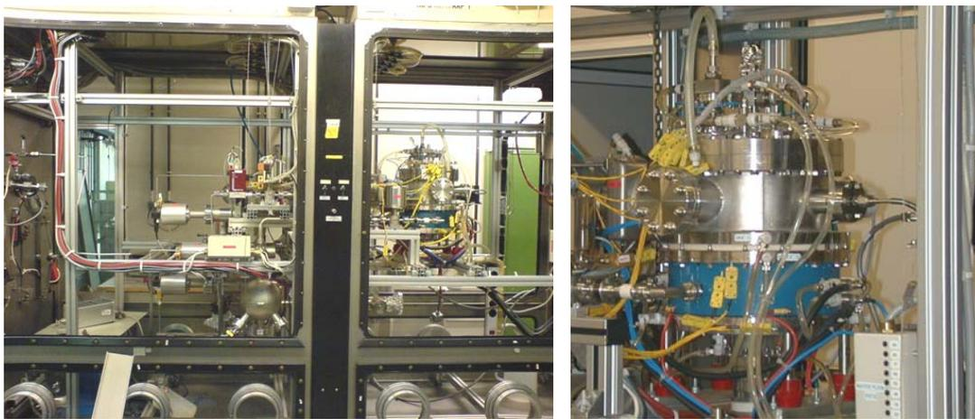
**FIGURE 1.** Pictures of the present status of the plasmatron facility VISION I in gloveboxes. Left: complete facility, Right: Plasma chamber.
