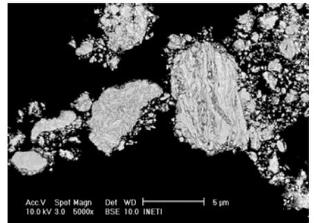
**FIGURE 2.** SEM/BSE pictures of W+nD powders milled for 2 h and 4h respectively (200rpm).
