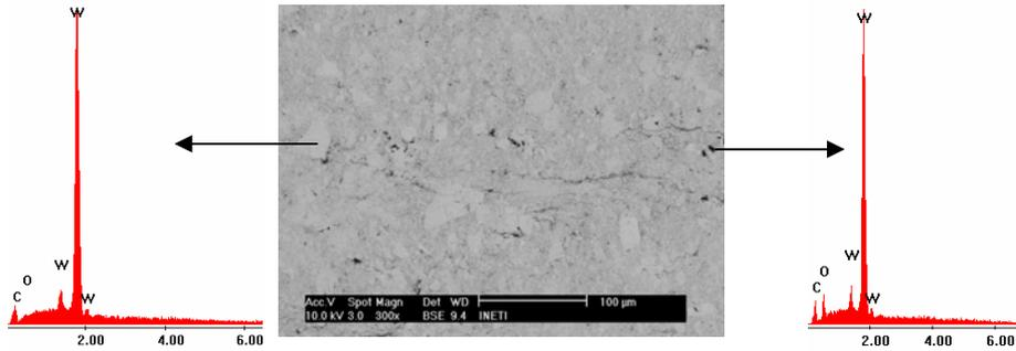
**FIGURE 3.** SEM/BSE image of W+nD subjected to MA (4 h at 200 rpm) and rolling at 800°C and respectively EDS chemical analysis.
