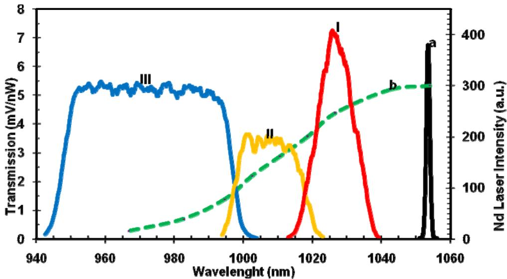
**FIGURE 4.** Thomson scattering general view with two vertical axes. Left axes, Optical Transmission: (I, II, III) Spectrometer channels transmissions (corresponding with the 1, 2 and 3 channels). Right axes: Optical emission intensity: (a) natural Nd:glass laser line and (b) typical laser Doppler broadening for 200 eV.
