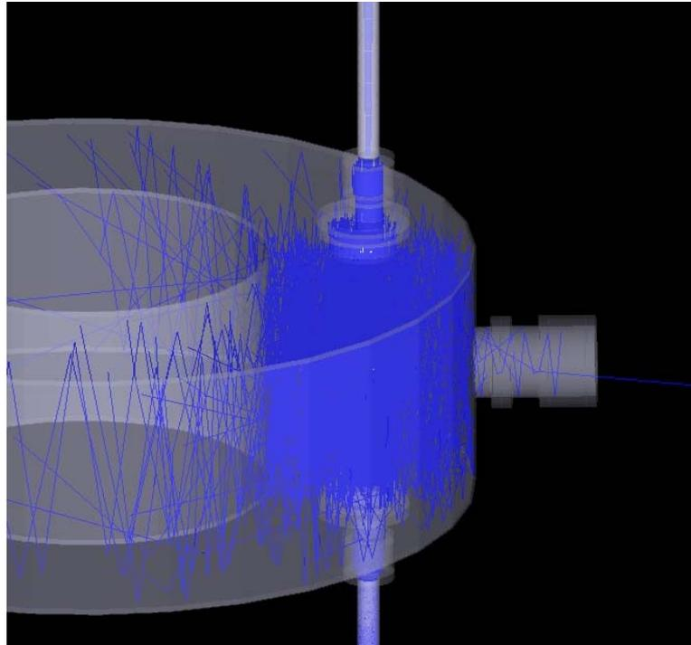
**Figure 5.** *Ray-tracing of the laser stray-light inside the vacuum chamber.*
