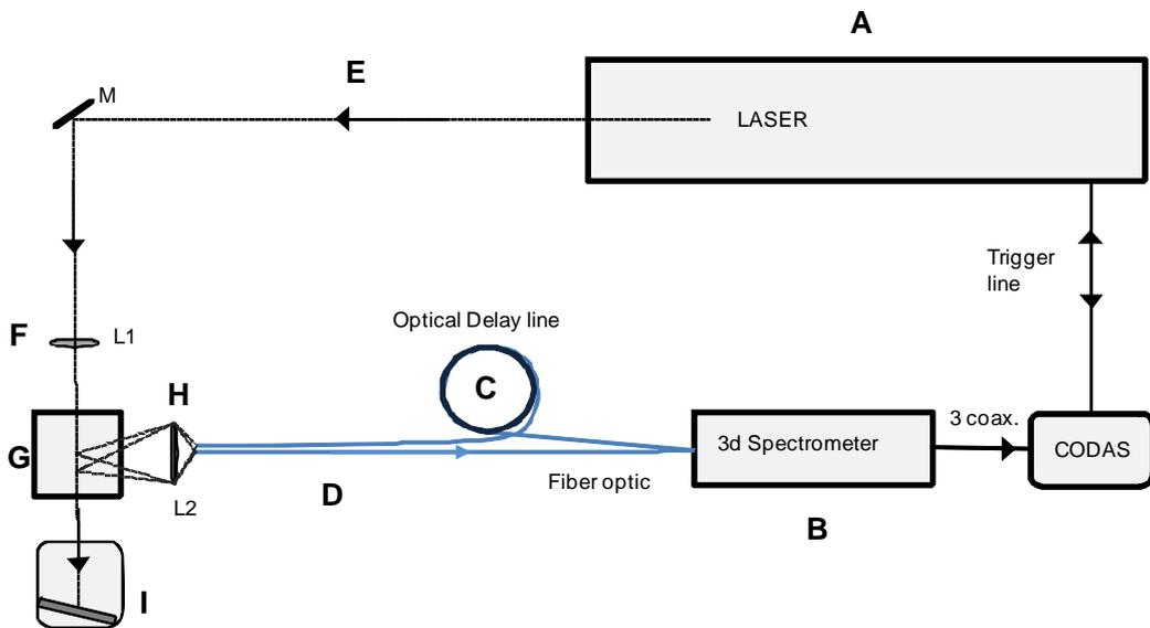
**FIGURE 1.** Lay-out of the TCABR Thomson scattering diagnostic. (A) Nd:Glass laser (PG38), (B) board with the spectrometers, oscilloscope and data acquisition PC, (C) optical delay lines, (D) optical fiber, (E) laser delivery system, (F) lens and input window to the vacuum vessel, (G) section of the tokamak, (H) collecting lenses, (I) main laser absorption dump.
