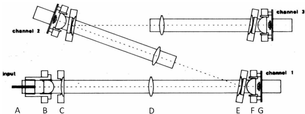
**FIGURE 3.** The Thomson Spectrometer Lay-out. Spectrometer made with three equal arms. Each arm has an interference filter that defines the spectral channel. (A) Fibers optic ends, (B) Collimating aspheric lens, (C) long range lens, (D) relay lens, (E) long range lens and interference filter, (F) focusing lens, (G) Si avalanche photodiode.
