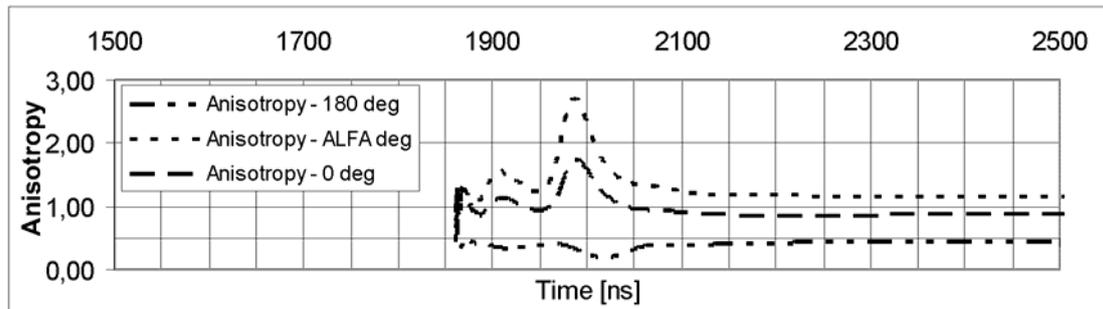
**FIGURE 7.** The exemplary results obtained during the measurements of the time-resolved neutron emission anisotropy.
