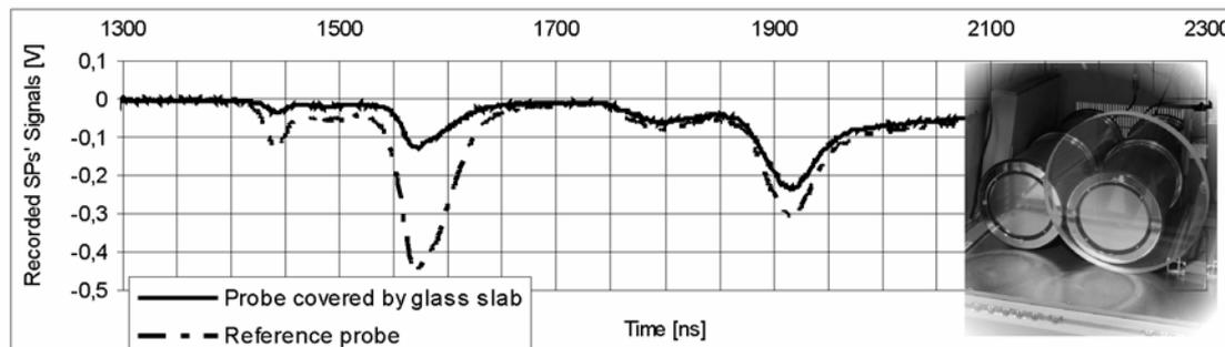
**FIGURE 8.** The investigations of neutron radiation scattering; The signals recorded from the reference as well as tested probe (covered by glass slab of 30 mm thickness) and the view of the arrangement.
