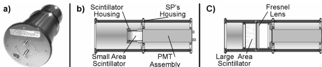
**FIGURE 1.** The scintillation probes FN-SP-1 type.
