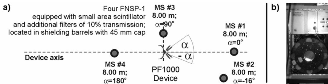
**FIGURE 6.** The four mobile stands arranged to carry out measurements of time-resolved neutron emission anisotropy: The simplified scheme of the mobile stands location at the experimental area (6a), The general view of the shielding barrel put into the mobile stand (6b).
