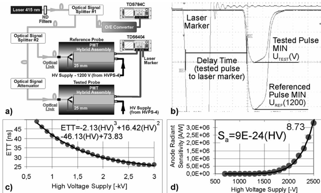
**FIGURE 4.** The investigations of the anode radiant sensitivity and delay time dependence on HV supply applied to the SP:
