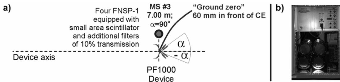
**FIGURE 5.** The relative calibration of the probes set: The location of the mobile stand in reference to the ground zero (5a), The general view of the four scintillation probes put into the mobile stand (5b).
