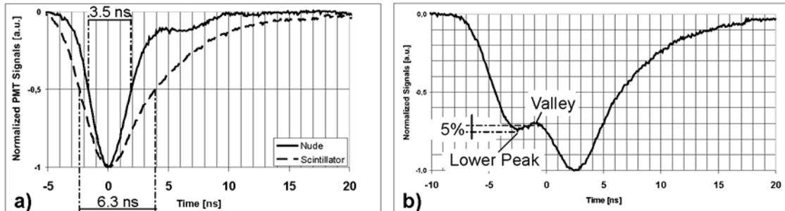
**FIGURE 3.** 3a) Comparison between the time response of the PMT itself (continuous line) and the time response of the scintillation probe (dashed line);
