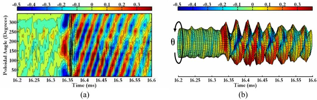
**FIGURE 5.** Mirnov raw signals in contour plot and 3D plot.
