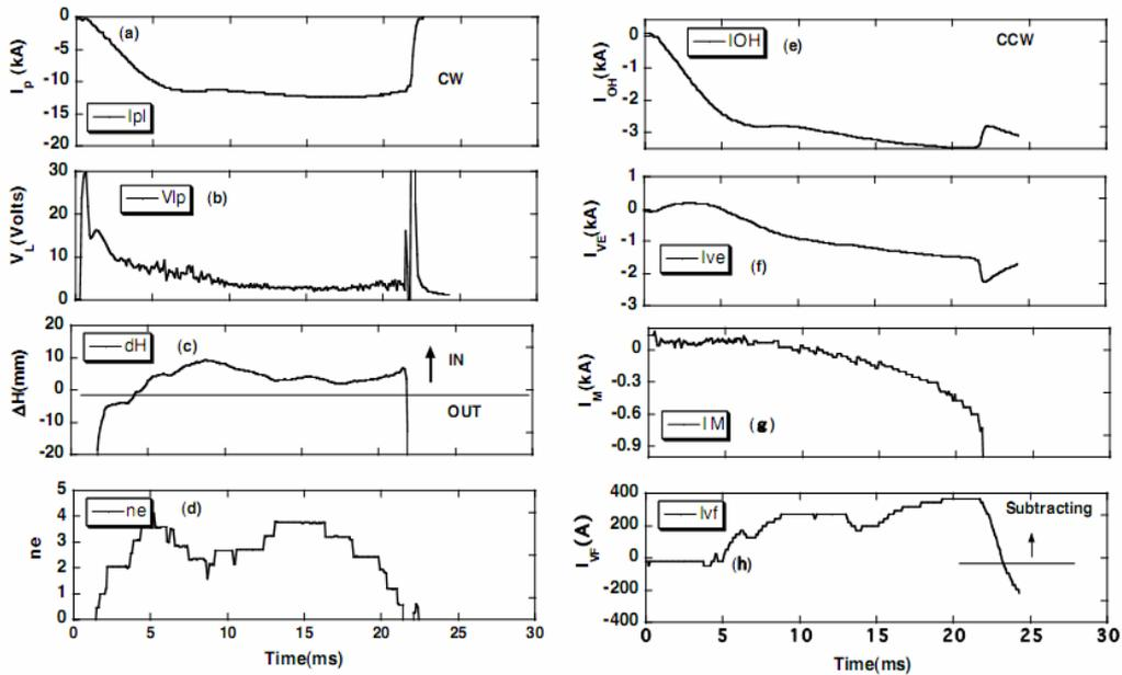
**FIGURE 11.** Experimentally observed current waveforms in the ST simulation (PF coil layout-1) in STOR-M. (a) plasma current, (b) loop voltage, (c) plasma position, (d) the line average density, (e) the outer OH coil current, (f) vertical coil current, (g) magnetizing current in the iron core, and (h) feedback coil current.
