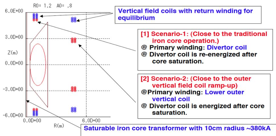
**FIGURE 1.** CTF PF coil layout for iron core operation.
