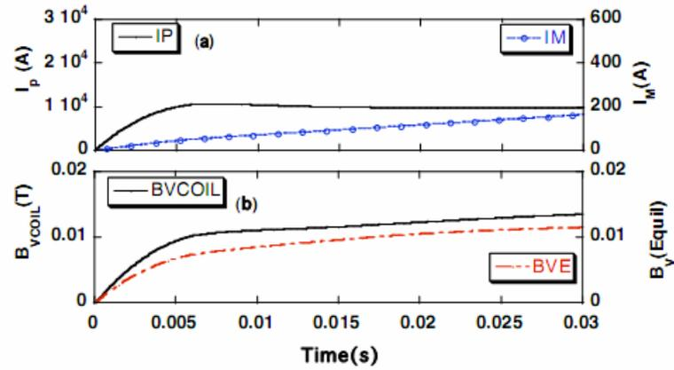
**FIGURE 10.** Numerically calculated current waveforms in the ST simulation PF coil layout-1 in STOR-M. (a) Plasma current (IP) and the magnetizing current (IM), (b) externally applied vertical field (BVCOIL) and equilibrium vertical field (BVE).
