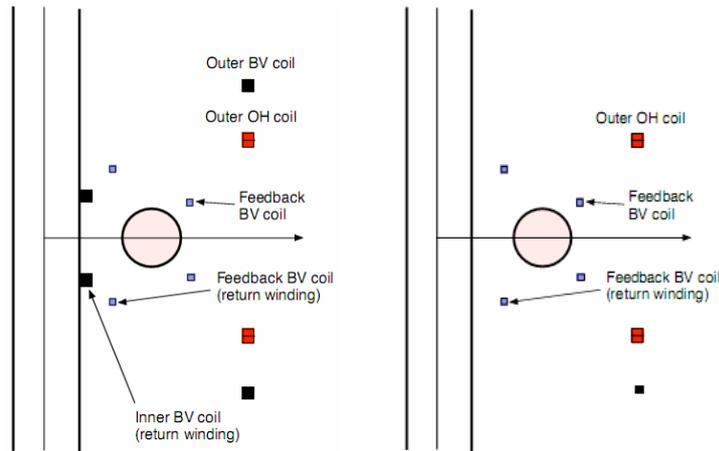
**FIGURE 9.** (a) ST simulation for the second operation scenario in STOR-M. (a) PF coil layout-1, (b) PF coil layout-2.
