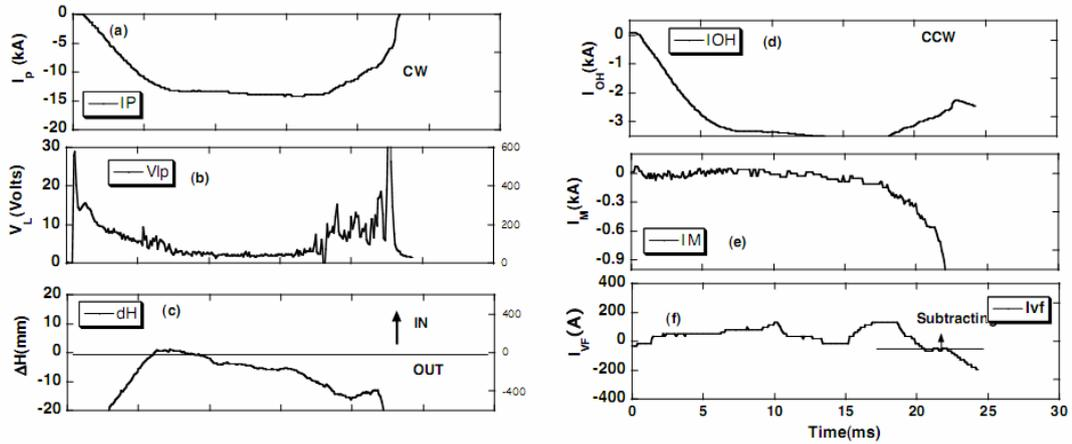
**FIGURE 12.** Experimentally observed waveforms in the ST simulation (PF coil layout-2) in STOR-M. (a) Plasma current, (b) loop voltage, (c) plasma position, (d) the outer OH coil current, (e) magnetizing current in the iron core, and (f) feedback coil current.
